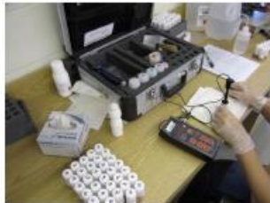
Drilled powder samples tested for chloride content
