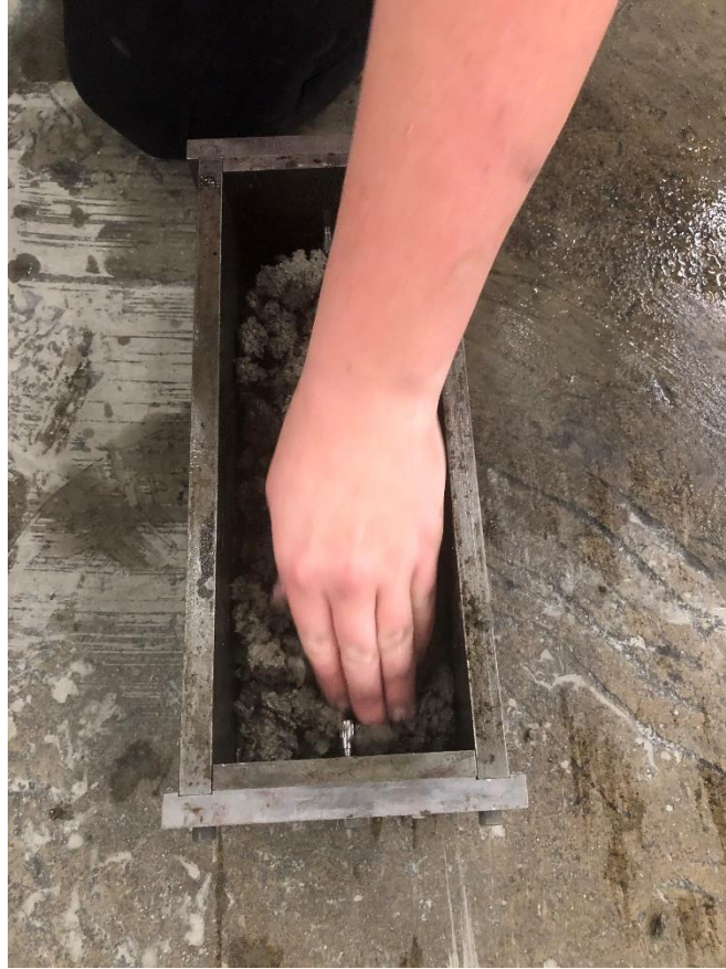
Figure 1: Preparation of beam specimens.
