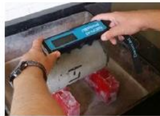
Resistivity testing for mixture acceptance
